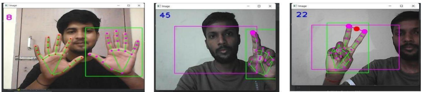
Fig 4: Hand Tracking, Mouse Movement & Mouse Zooming Recognition
