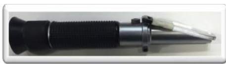
Fig.5 Image of a typical hand refract meter used to measure fluid concentration
