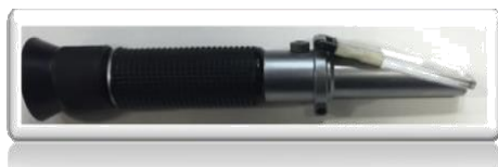
Fig.5 Image of a typical hand refract meter used to measure fluid concentration
